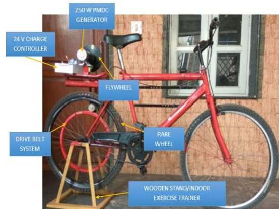
Fig 33: Represents Hardware model of an Off-Grid Eco-friendly Green Energy Harvesting (EH) Flywheel Based Bicycle Generator.
