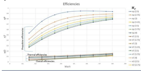
Fig. 17 Turbojet performance vs Mach: efficiency
